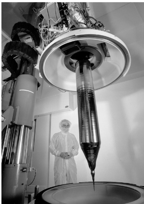
Fig. 2.4. Crucible-grown modern dislocation-free silicon monocrystal (courtesy Wacker Chemitronics)
