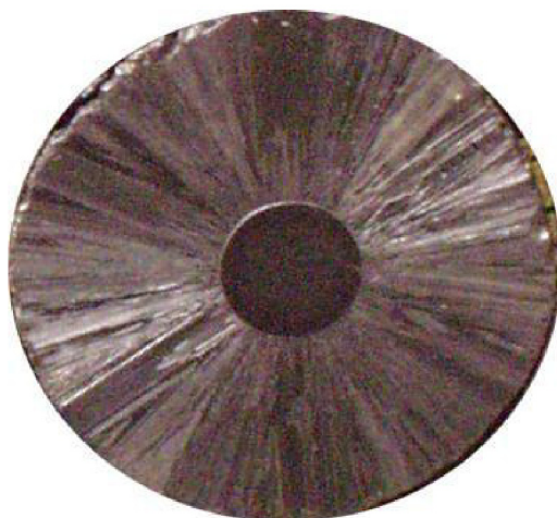
Fig. 2.3. Cross section of a thickened silicon rod. The monocrystalline center is surrounded by a polycrystalline CVD layer
